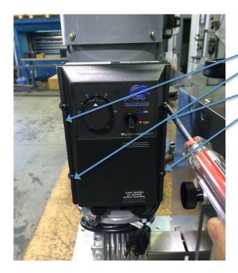
Unscrew 4 screws and remove the drive cover.
