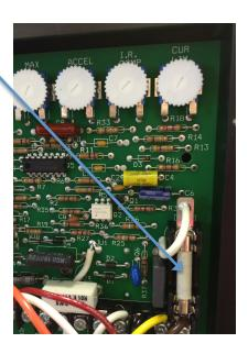
Replacement Fuses specifications: These fuses can be bought at a local electrical store. 250V FA 3ABPp- Free 10A
